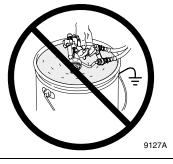
Do not wipe the gun with a cloth soaked in solvent; ring out the excess.
